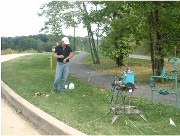
*Field setup of the Syskal DC resistivity equipment manufactured by Iris Instruments*
