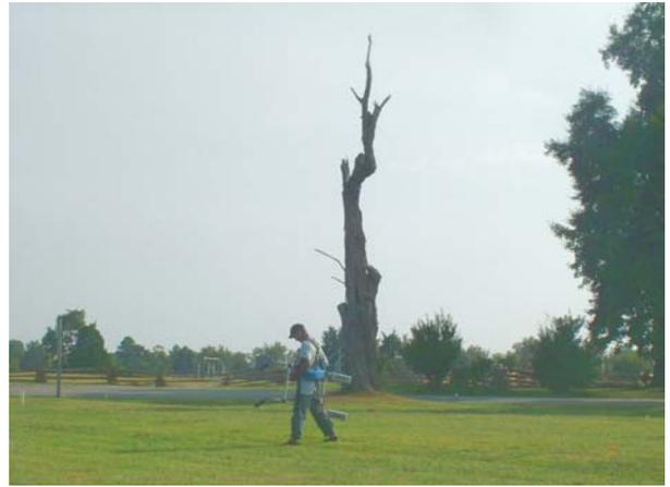
*Magnetic surveying with an EG&G G858G gradiometer at the "Triangle" site*
